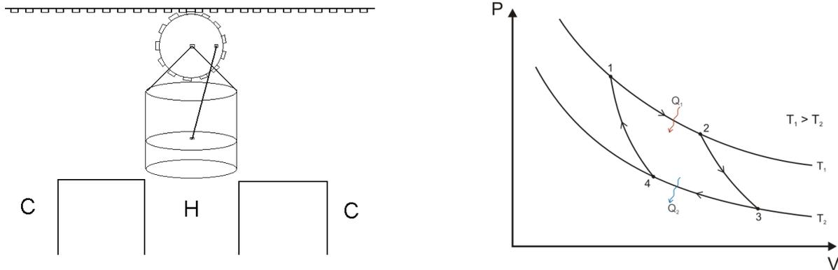
In this diagram, the gas is stored in a cylindrical tank that is free to slide on a track above an infinite sequence of alternating hot and cold reservoirs with insulating barriers between them. The expansion and compression of the gas is mechanically linked to the motion of a massive gear that forces the tank-gear apparatus to crawl along the strip at the top. We assume that the whole system is frictionless and that everything besides the gear is massless.
